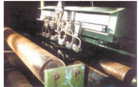
Testing with oscillating probes
